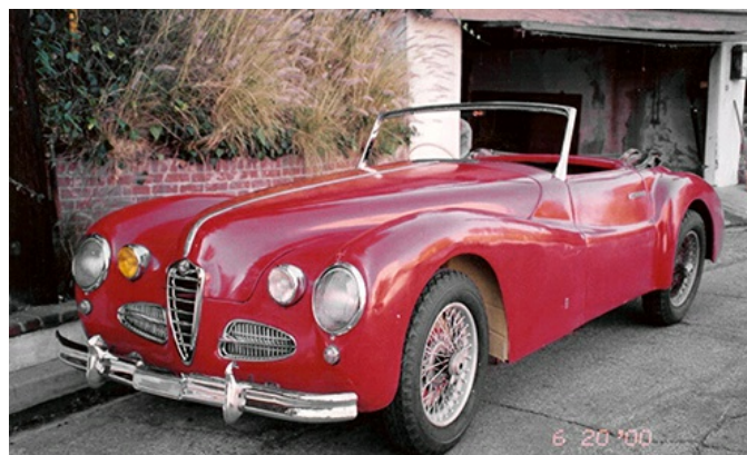
1943 Alfa Romeo 6C 2500 Super Sport Cabriolet in California in 2000 with the later type 1900 grille and extra headlights added in 1953. Photo courtesy of David Cooper.
